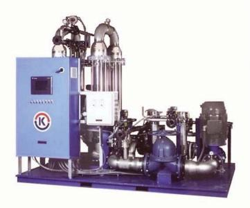
KEMCO's Ceramic Microfiltration System is a cost effective way to achieve a high recycle rate for industries that require large amounts of process water. KEMCO's CMF System removes suspended and emulsified contaminants from wastewater, without the addition of treatment chemicals. Through the use of ceramic elements with porosity of less than 1 micron, wastewater is cleansed to a recyclable quality.
