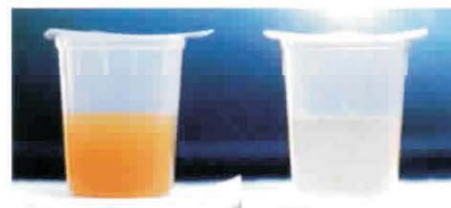
Comparison of: (left) wastewater treated with DAF system, and (right) wastewater treated with ASH system.
